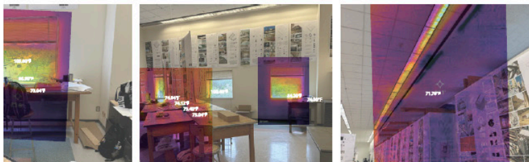
Figure 3. Examples of data collection and analysis during the post-occupancy evaluation project. Students study occupant comfort and satisfaction (occupant survey), thermal and visual patterns in spaces (spot measurements and datalogging), and human comfort (thermal imaging and interviews). Images taken or created by level 1 MARCH students in May 2023.
